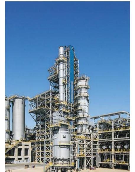
RFCC공정(Residue Fluidized Catalytic Cracking)
